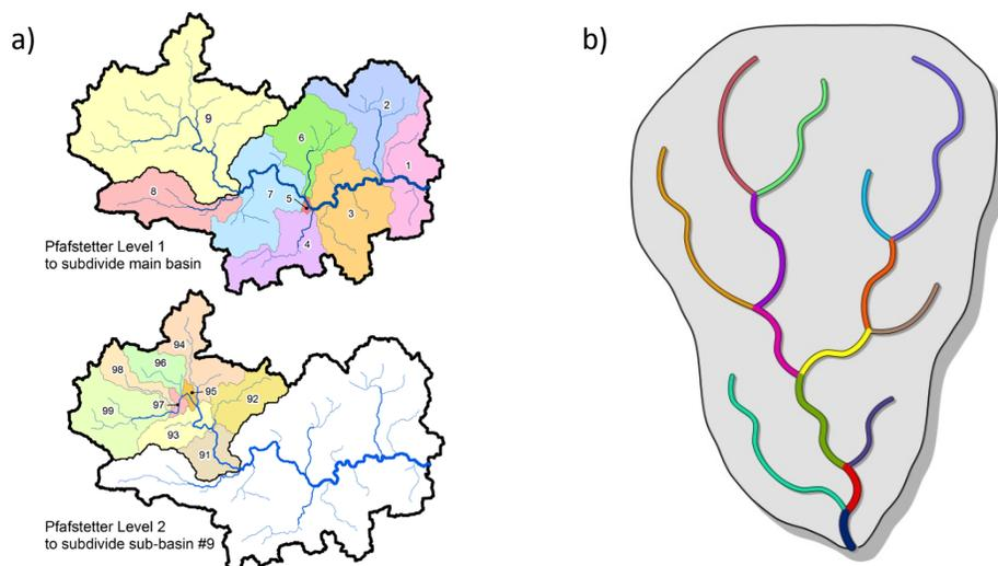
**Figure 1: Overview of Pfafstetter sub-basin coding scheme used in BasinATLAS (a); and river reach concept used in RiverATLAS (b). Sub-basins are nested within 12 hierarchical levels. A river reach is defined as a stretch between two tributaries, or between the start/end of the network and a tributary.**
